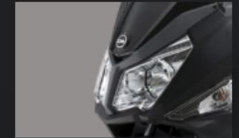
Dual headlights 35W/35W and LED position lights
